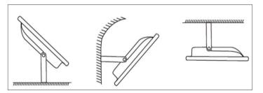
Install the LED flood lights in the ground, wall, and ceiling
